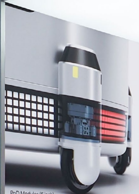
Pro Modules (6 inch) - Intelligent steering, braking, in-wheel electric drive, and suspension
